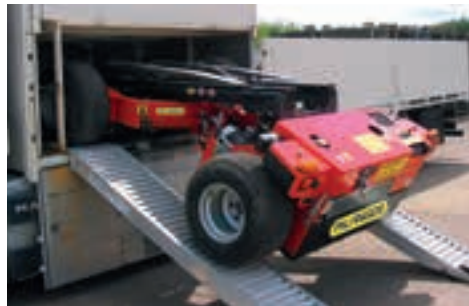
ON TOP - DRIVEN ONTO LOAD PLATFORM USING RAMPS
