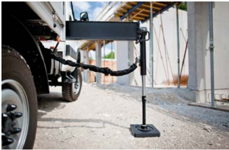
STABILIZER SYSTEM FOR OPTIMUM STABILITY
