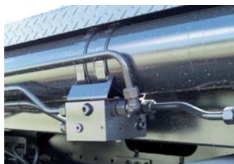
Check valves on each hydraulic cylinder
