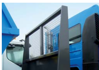
Protective wall between cab and container
